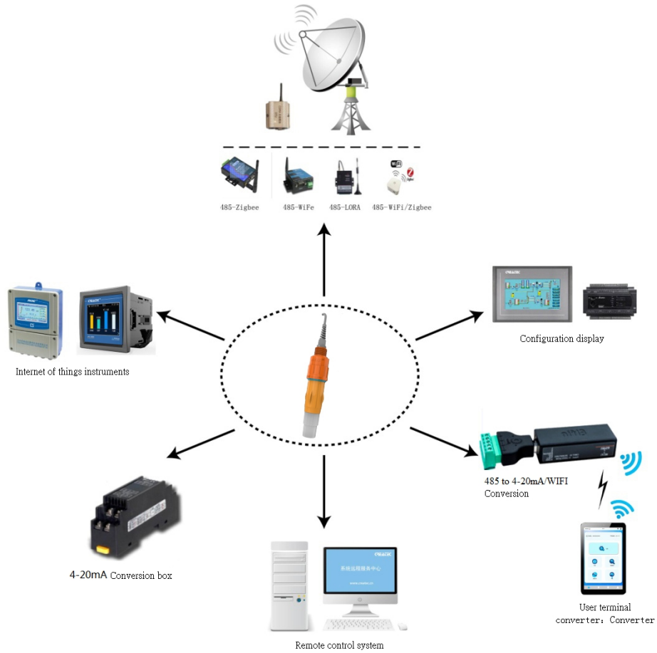
Figure 4.1 Multiple display modes of data acquisition terminal
